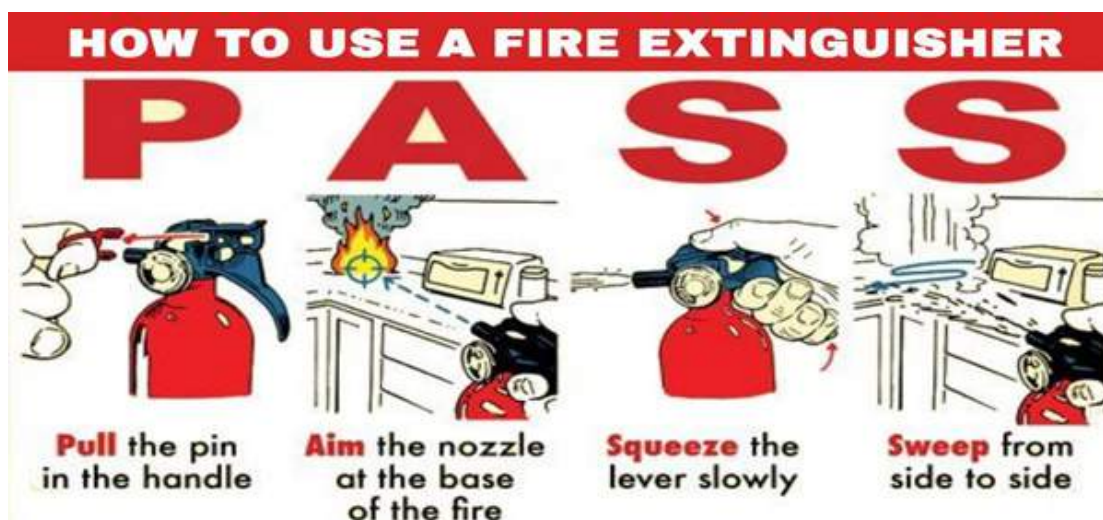
Fig. 6.7.2: Pass technique for Fire Extinguisher use
