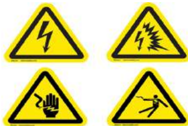
Fig. 6.3.2: Electrical hazard symbols
