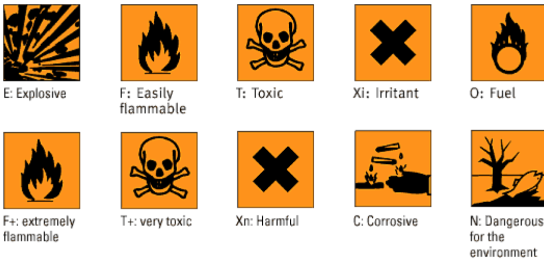
Fig. 6.13.2: Chemical hazard safety signs
