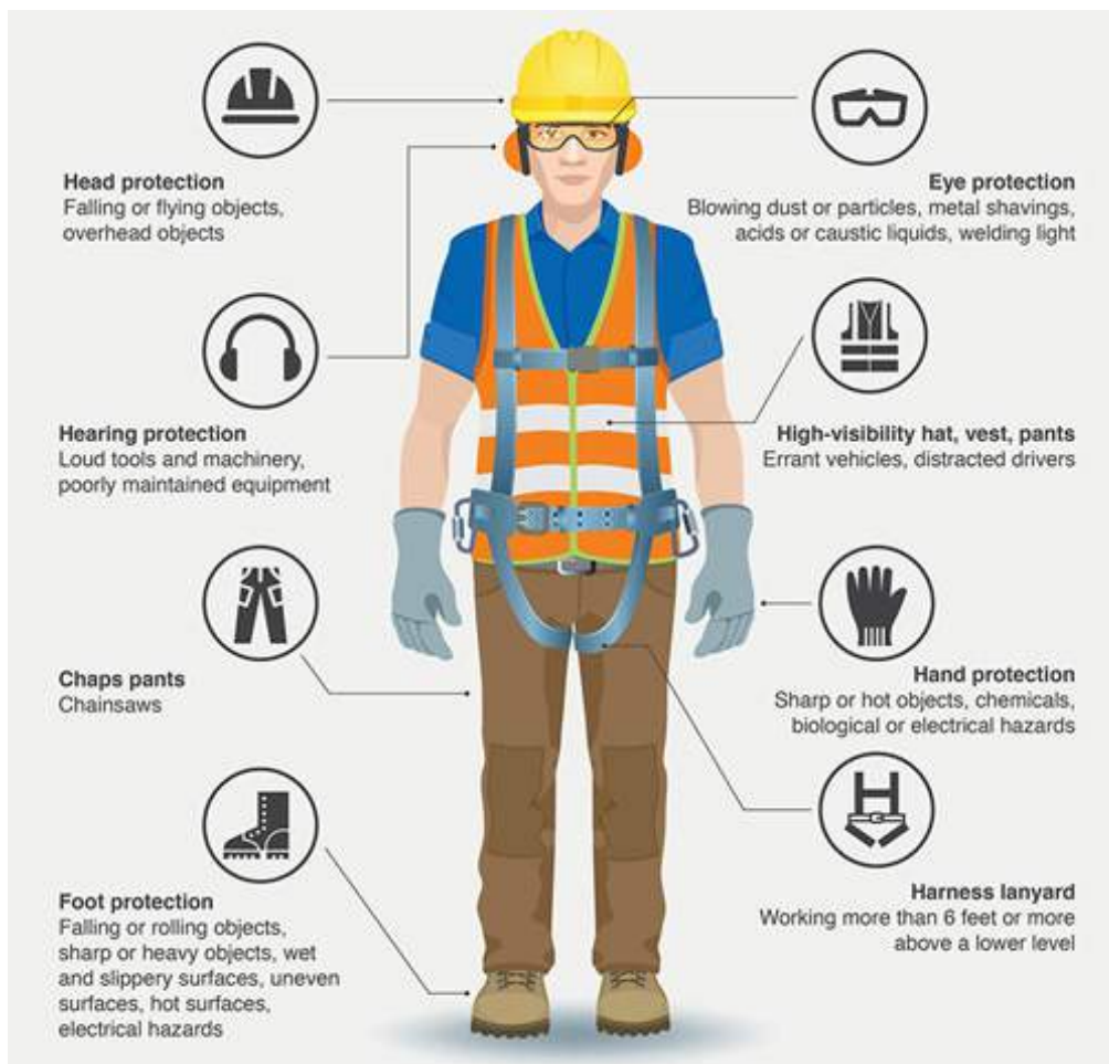
Fig. 6.4.1: The usage of personal protective equipment
