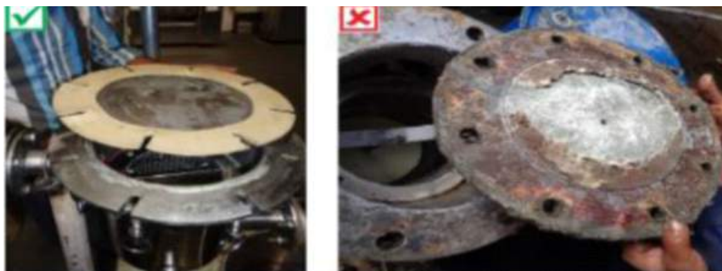
Fig 4.5.4 Usage of appropriate food grade gasket
