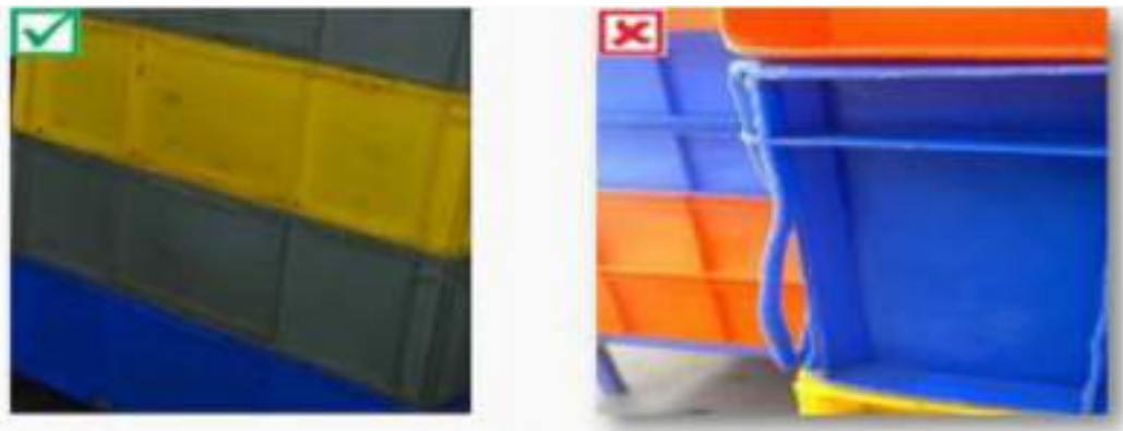
Fig 4.5.3 Damaged containers(source of foreign matter contaminations) should not be used inside the process
